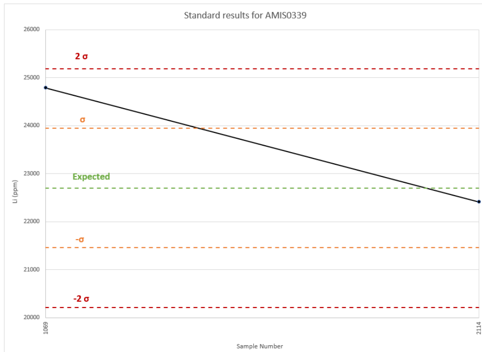
Figure 11-2 – Standard Sample Analyses Results for the 2017–2018 Batch with Standard AMIS0339
